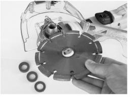
Install wheel. Insert appropoiate spacers to adjust • /center wheel in the shroud for best performance. Make sure cut wheel is seated flat.
