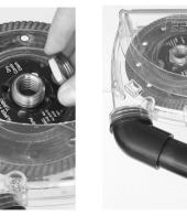
Insert hose to port. Use • releasable tie to secure hose & electrical cord together.
