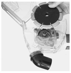
Follow Installation steps and install crack chasing wheel.
