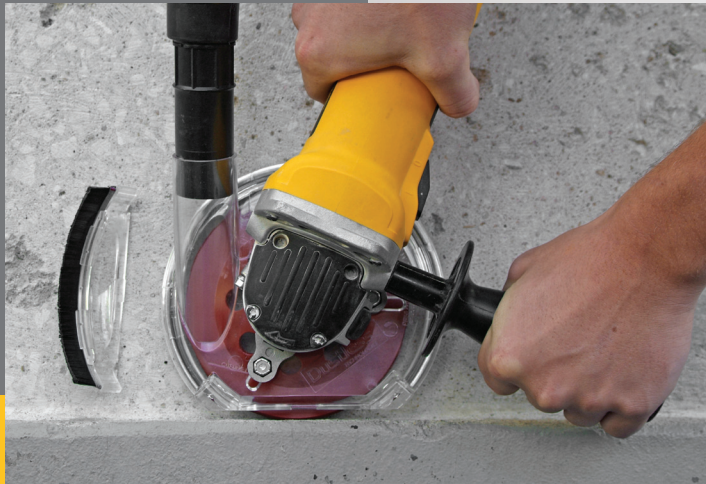
Removable lip enables grinding against a wall.
