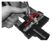
5. Ensure the front rubber dust shield is properly positioned within both the upper blade guard of the saw and the blade opening in the shroud. The shield should form a "C" channel in front of the blade.
