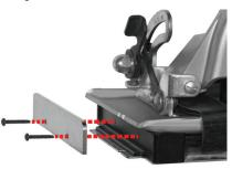
Position the saw as far back on the shroud as it will sit. Use the included zip tie to fasten the saw's depth guide arm to the hose port of the shroud to restrict the saw from moving forward. Position the saw against the left wall and continue with step 4 of installation.
