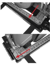
4. Firmly fasten both cinching straps around the shoe plate of the saw. Keep the buckle anchored to the edge of the shoe plate, as shown.
